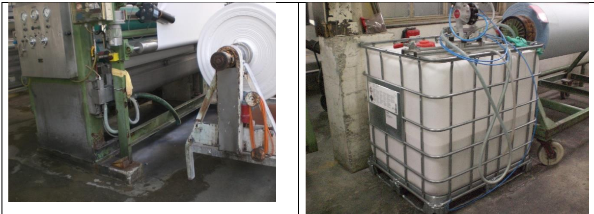
Figure 1: On the left, the photo shows the padder of a stenter and on the right an intermediate bulk container (IBC) equipped with a pump and pipes to manually empty the padder (Photos: Dr. Harald Schönberger)
